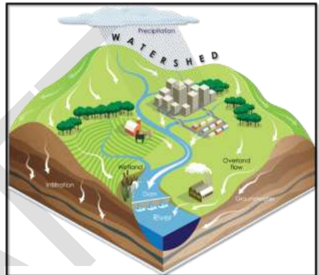
Figure 1-2. Stormwater runoff in a watershed.
